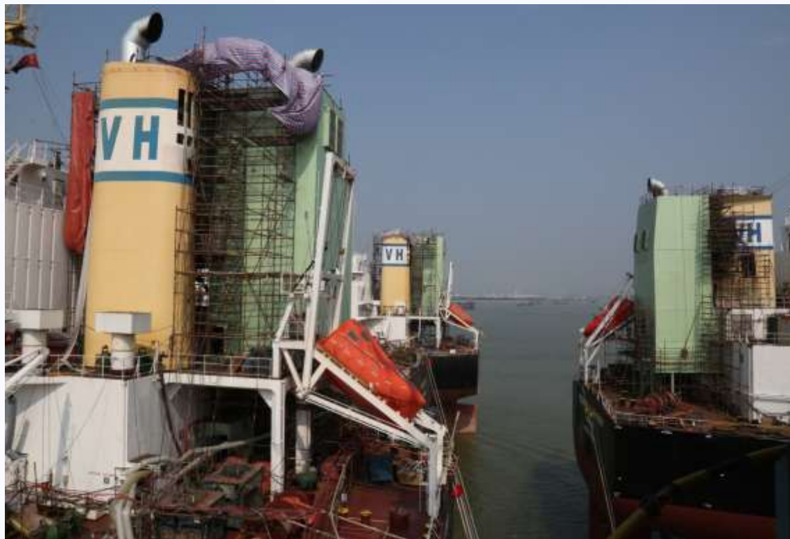
Scrubbers installed on board MV Venus Horizon, MV Venus History and MV Pedhoulas Cherry.
